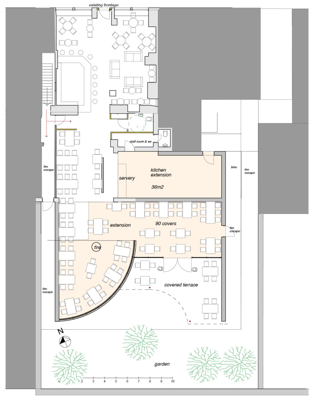
Note: area of extension shown tinted new roofs drained to soakaway
