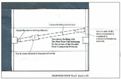
Fig 12 - route of extract duct through loft of flat at no227
