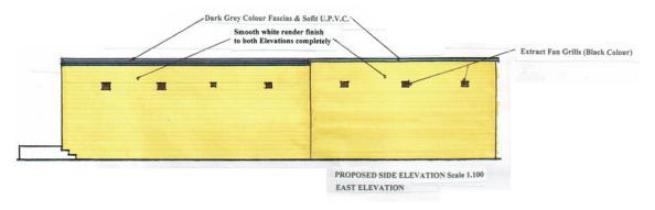
Figure 4 East facade showing the location of the extract grills
